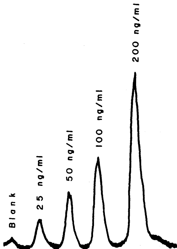
Figure 2—Chart tracing for a blood standard curve.
